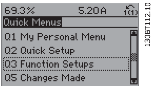
Illustration 6. 4: Step 3: Use the up/down navigation keys to scroll down to Function set-ups. Press [OK].
