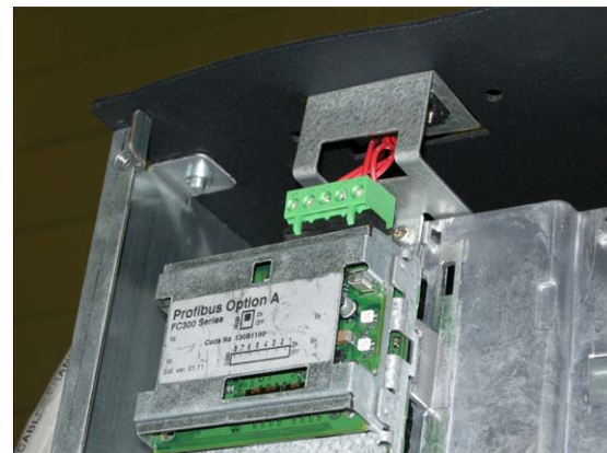
Illustration 4. 16: Top connection for fieldbus.
